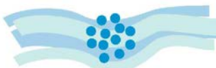
The Mod Media system strips away particles as small as 70 microns, (an average grain of beach sand is 100 to 2000 microns in diameter).
